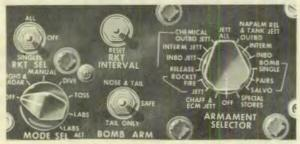
The square shape and location in the cockpit requires that the pilot scrutinize the switch closely to insure its correct position. Action has been initiated to replace the square type switches, but in the meantime double check before you press the utton.
