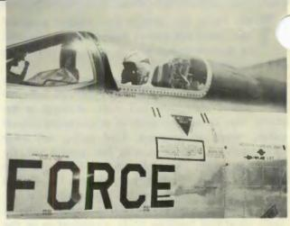
All pilots pulling mobile control should glance at these photographs of the F-105. In the picture on the left the canopy is unlocked and will come off in flight unless someone...you...calls it to the pilot's attention. On the right, the aircraft is clear and ready to go. We deliberately failed to include the usual set of arrows pointing out the difference, since they won't be there if the real thing comes your way.
